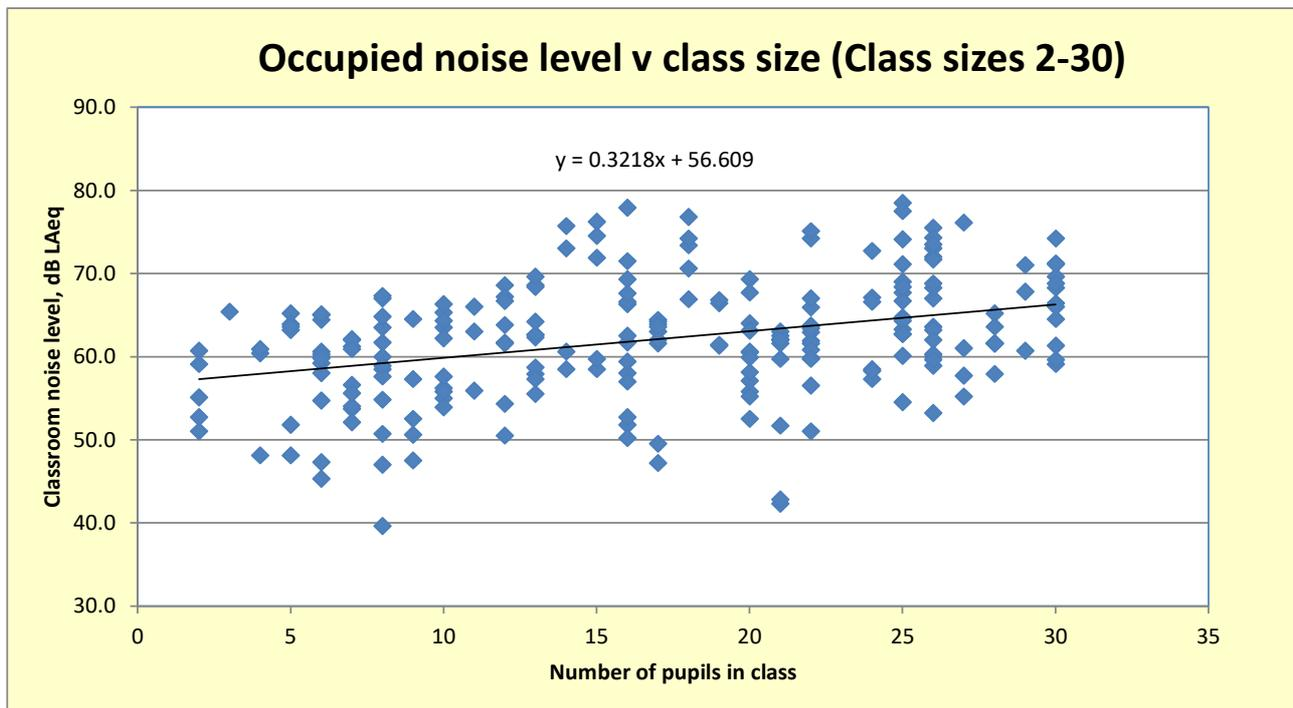
Figure 2: Comparison of results uncorrected for reverberation time
